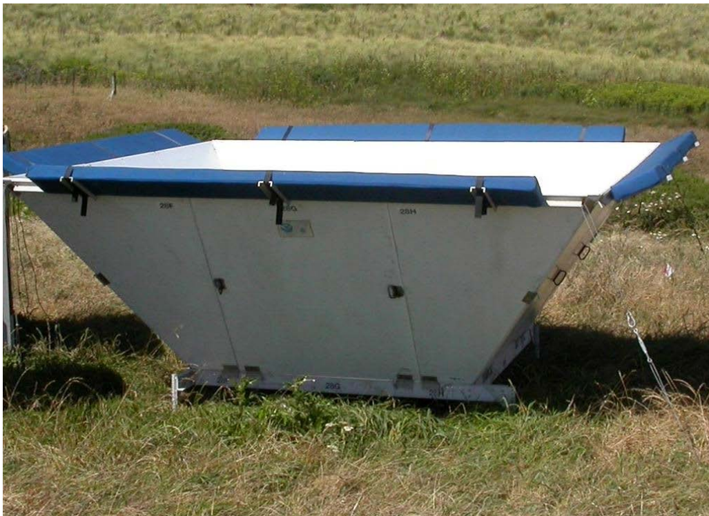
915 MHz phased array wind profiler
