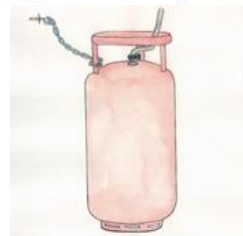
Fig 31. Anchoring Gas Cylinder
